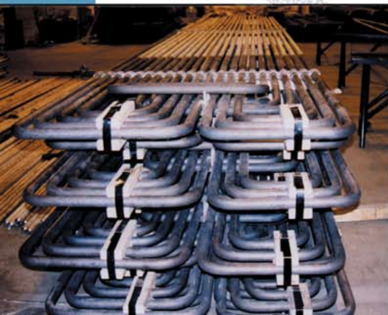
◀ Reheaters manufactured with a complete material upgrade that includes both stainless and inconel
